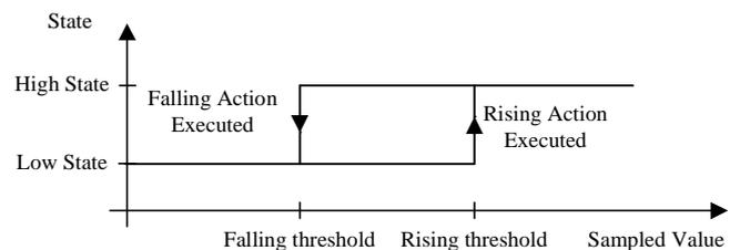
Figure 10: Threshold Operation.
