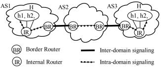
Figure 1: Two-tier QoS Signaling
