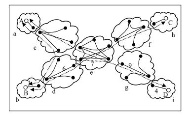
Figure 3. Multi-AS connections and the associated paths
