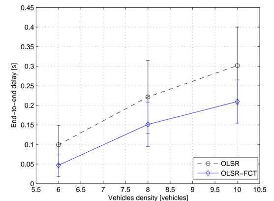
FIGURE 3: OLSR and OLSR-FCT performance evaluation: end-to-end delay (s).
