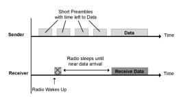
Figure 1: MH-MAC asynchronous broadcast transmission.
