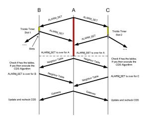
Figure 2: ALARM-SET flooding protocol example.
