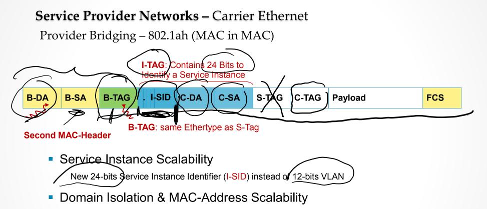
Encapsulate Customer MAC frames at the edge of the network into Backbone MAC frames: New MAC header
