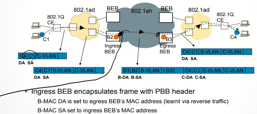
I-SID determined based on S-VLAN & B-VLAN determined based on I-SID
